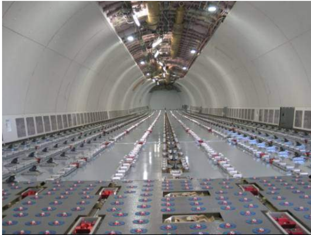
The versatile main deck of the A330F facing AFT showing the enhanced cargo loading system
